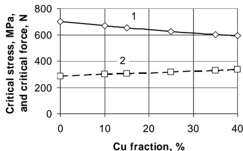
Fig. 2. Dependence of critical axial stress (1) and critical tensile force (2) on cross-sectional fraction of Cu layer. Calculations by FE model;
