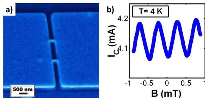
Fig. 1. a) Scanning electron microscopy picture of a Dayem bridge nanoSQUIDs, consisting of two nanowires in parallel connecting two wider electrodes. b) Critical current modulation of a nanoSQUID measured at 4 K as a function of an externally applied magnetic field.
