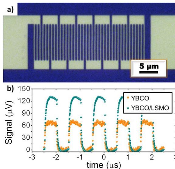
Fig. 3. a) Optical picture of 10  $\mu\text{m}$  long YBCO/LSMO nanowires, embedded in a configuration covering a large area, suitable for photodetection experiments. b) Voltage responses to optical laser pulses ( $\lambda = 1550 \text{ nm}$ ) measured at 5 K on two devices with the same geometry, but employing respectively bare YBCO and YBCO/LSMO nanowires.
