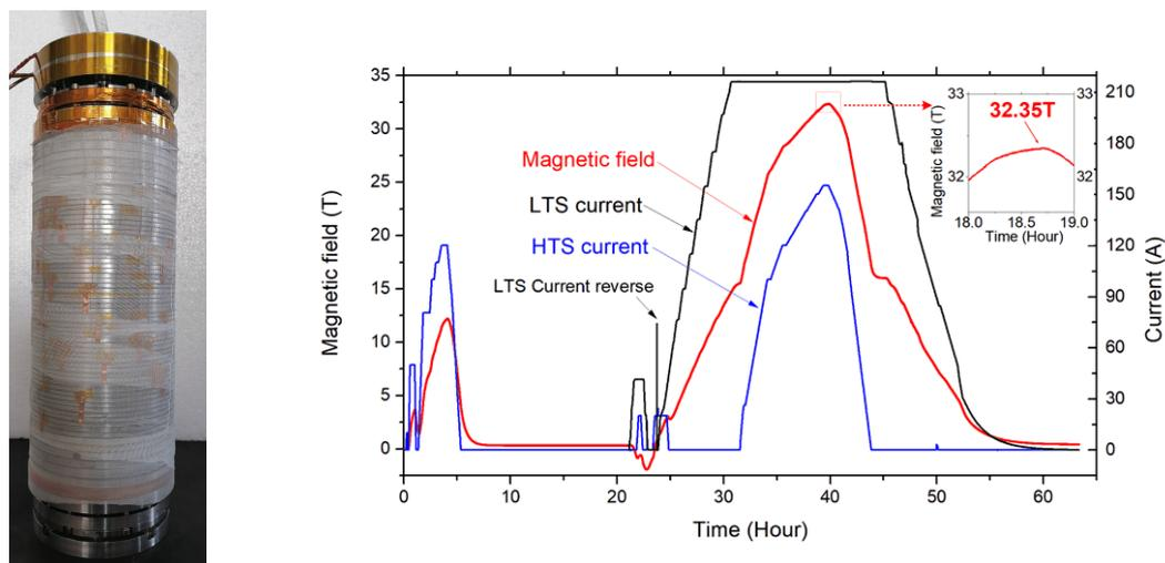
**Fig.1.** The REBCO insert (left) and the excitation process at 4.2 K (right). During the excitation process, the current direction of the LTS magnet was changed one time as shown in the figure, since the direction of the magnetic field generated by the LTS magnet was against the direction of the magnetic field generated by the HTS insert.
