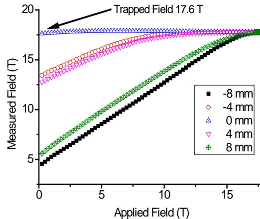
**Fig. 2.** The field measured at the interface between the two samples in the stack by an array of Hall probes (distances indicated are from the centre of the sample) as the magnetising field was ramped down. [Reproduced from [1] under the CC-BY license]
