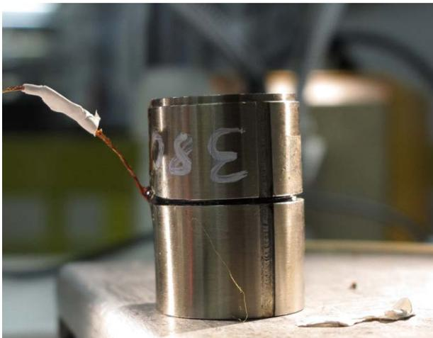
**Fig. 1.** The assembled stack of two GdBCO bulk samples, each of diameter 24.15 mm and height 15 mm. The samples were reinforced with a ring of 3 mm thickness fabricated from 304 Stainless Steel.
