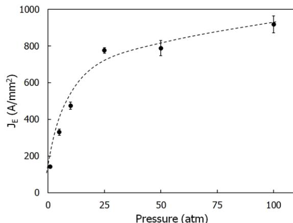
Fig. 3. Evolution of the engineering current density as a function of the OP pressure applied during the heat treatment. The partial pressure of oxygen is kept constant at 1 atm the entire heat treatment.
