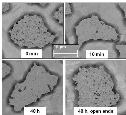
Fig. 2. Cross section of Bi-2212 filaments from sealed wires heat treated at 821°C for 0 min, 10 min, 48 h and 48 h with open ends. The OP was set at 50 atm with 1 atm of O<sub>2</sub>.
