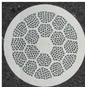
Fig. 1. Cross section of an 0.8 mm in diameter Bi-2212 round wire made by OST.
