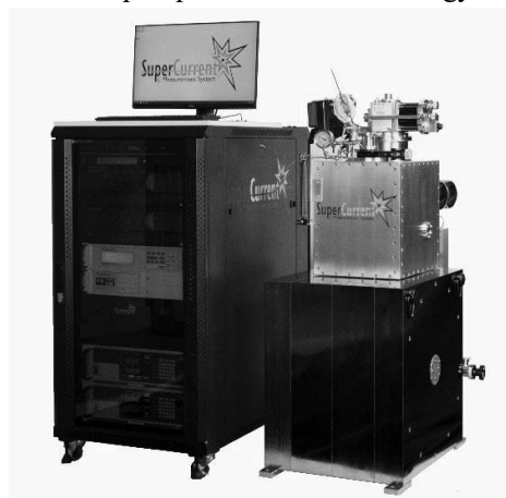
Fig. 1 ‘SuperCurrent’ I_c characterization system.
