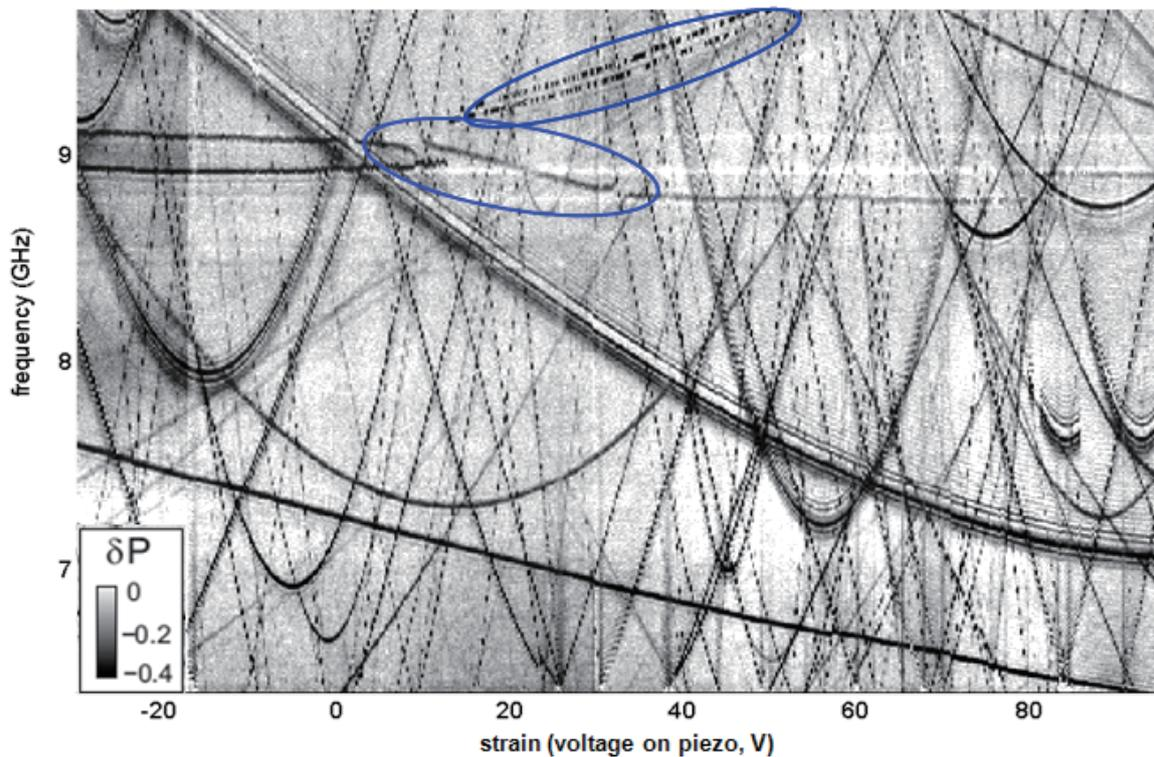
Figure 1: TLS spectroscopy, showing the resonance frequencies of strain-tuned individual TLS as dark traces. Encircled are anomalies which provide evidence of mutual coupling between TLS.
