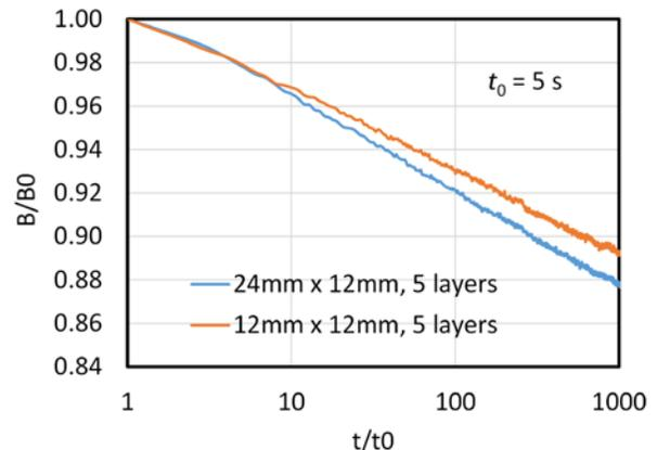
Fig. 4. Flux creep data for a square and rectangular stack of tapes magnetized by field cooling at 77.4 K. The initial trapped field  $B_0$  is 74 mT and 64 mT for the rectangular and square stack respectively.
