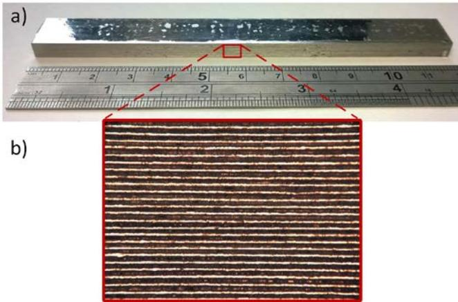
Fig. 2. (a) 12 mm by 120 mm by 5.2 mm stack of 60 tape layers bonded together by heating and compressing the stack whose layers have been pre-coated solder. (b) Zoomed image showing uniformity of layers from the side of the stack.
