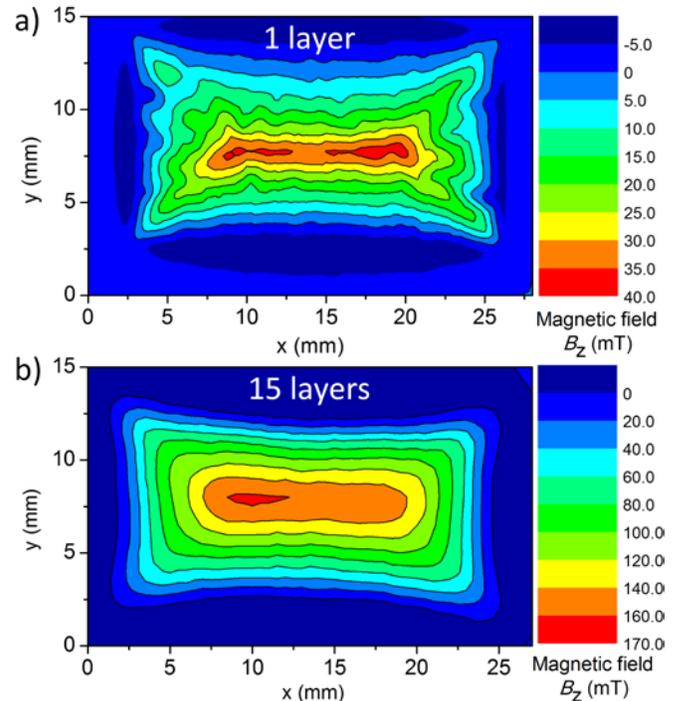
Fig. 3. (a) Trapped field for a single layer and (b) 15 layer stack, composed of 12 mm by 24 mm tape rectangles. Magnetized using field cooling at 77.4 K showing a relatively symmetric profile. The field was measured 0.8 mm above the sample surface in both cases.
