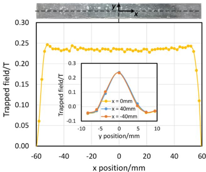
Fig. 8. Trapped field profile for a 60 layer self-supporting stack, with layers soldered together. Magnetized using a pulsed field at 77.4 K. The average center field 0.8 mm above surface is 0.235T.
