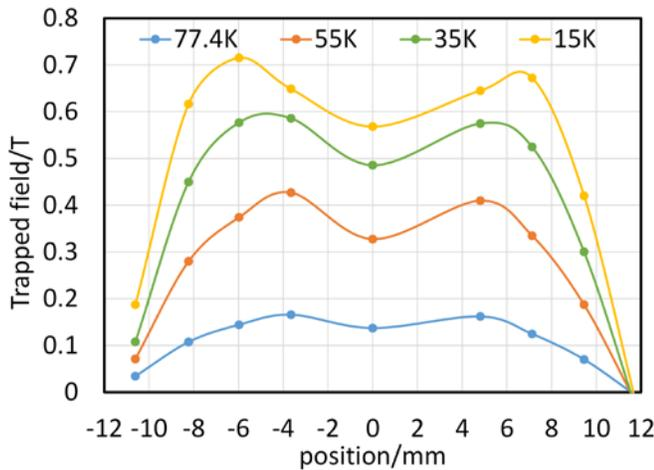
Fig. 5. Trapped field profiles for 15 layer stack composed of 12 mm by 24 mm tape layers. Pulsed field magnetization was used with a sequence of pulses applied at each temperature stage followed by cooling to the next temperature stage, allowing the maximum possible trapped field for pulsed magnetization to be established.
