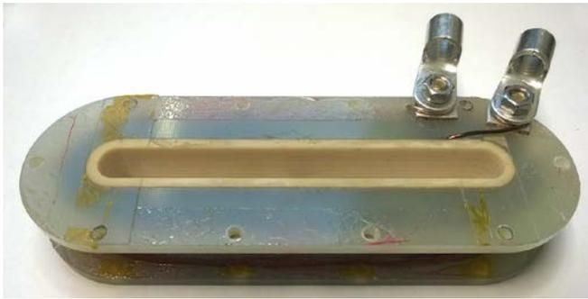
Fig. 7. Race track shaped pulsed field coil used to magnetize the long rectangular stacks of tape. Made from copper wire with internal glass fiber reinforcement. Pulses delivered had a duration of 29 ms.
