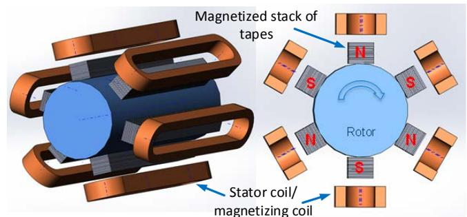
Fig. 1. Conceptual drawing of a motor using rectangular stacks of tapes as field poles on the rotor, magnetized by race-track copper coils on the stator which also act as the motor's stator coils during operation.
