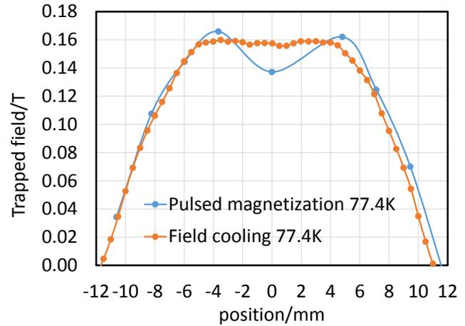
Fig. 6. Comparison of the trapped field profiles for the 15 layer, 24 mm by 12 mm stack, resulting from field cooling and pulsed magnetization at 77.4 K. Although pulsed magnetization gives a similar peak trapped field, it gives rise to a dip in the central field.
