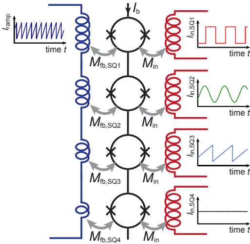
Fig. 3. Schematic circuit diagram of a four-channel MHz frequency-division SQUID multiplexer based on the dc-SQUID readout scheme introduced within this work. The  $I_{in,SQ_i}$ -vs.- $t$ -plots close to the input coils (red) of the SQUIDs illustrate the test signals used for generating the data shown in Fig. 4.
