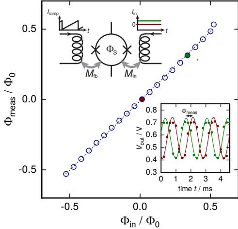
Fig. 1. Reconstructed magnetic flux change  $\Phi_{\text{meas}}$  versus the applied magnetic flux change  $\Phi_{\text{in}}$  using the dc-SQUID readout scheme discussed within this paper. The upper left inset depicts the used readout configuration and the lower right inset displays the measured flux-to-voltage SQUID characteristic for  $\Phi_{\text{in}} = 0 \Phi_0$  (red line and dots) as well as  $\Phi_{\text{in}} = 0.35 \Phi_0$ .
