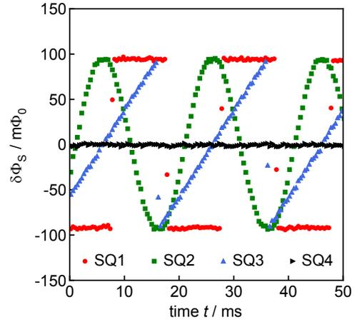
Fig. 4. Measured magnetic flux change  $\delta\Phi_S$  versus time  $t$  in channels SQ1 to SQ4 of the four-channel MHz frequency-division SQUID multiplexer introduced within this work. The test signals that were applied to the input coils of the different channels are illustrated in Fig. 3.
