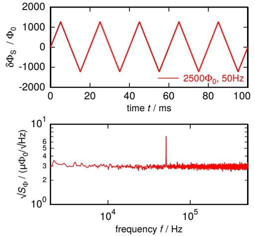
Fig. 2. **a)** Reconstructed magnetic flux amplitude  $\delta\Phi_S$  versus time  $t$  for a  $2500 \Phi_0$  (peak-peak) triangular signal with a repetition rate of  $50 \text{ Hz}$  and **b)** measured flux noise spectrum of the SQUID setup read out using our readout approach in the absence of any input signal. For the measurement, a flux ramp with an amplitude and repetition rate of  $4.2 \Phi_0$  and  $1 \text{ MHz}$  were used.
