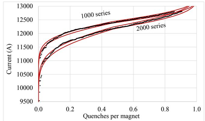
Fig. 9: Training (second quench) in 2000 series and Gaussian fit with 30% lower  $\sigma$  in the right part.
