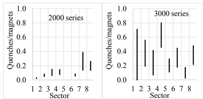
Fig. 4: Probability to quench before 11080 A during 2015 commissioning in the 2000 series (left) and in the 3000 series (right) split by sector.
