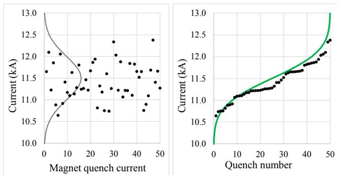
Fig. 2: Left: Example of a Gaussian distribution (grey curve), extraction of 50 quenches (dots): Right: reordering of quenches giving the training of a string of 50 magnets (dots) and integral of the Gaussian (green curve).
