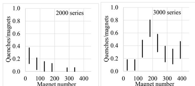
Fig. 5: Probability to quench before 11080 A during 2015 commissioning in the 2000 series (left) and in the 3000 series (right) split along the production in batches of 52 magnets.
