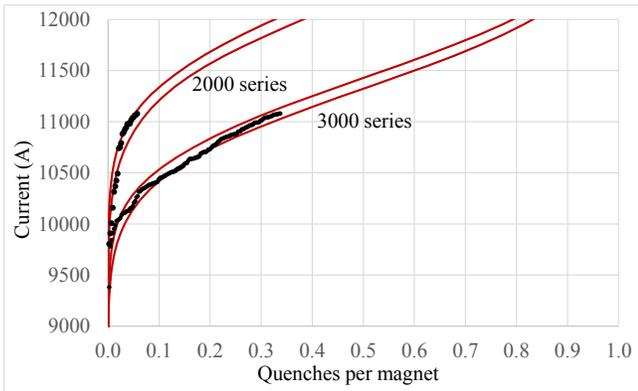
Fig. 6: Training in 2015 (first quench) in 2000 and 3000 series, and Gaussian fit with two sigma error.
