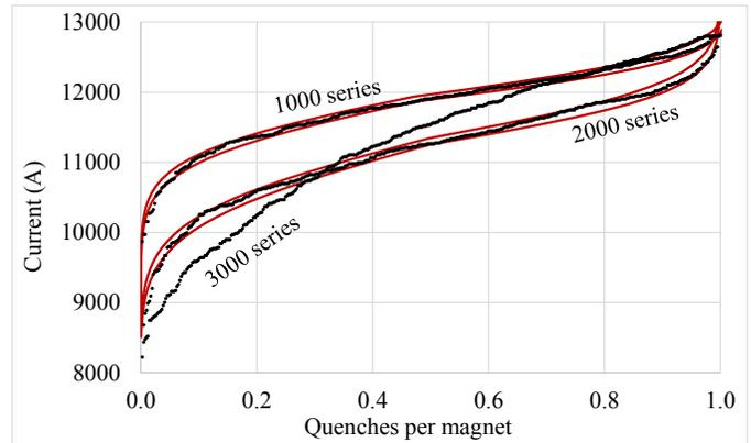
Fig. 8: Training (first quench) in 1000, 2000 series and Gaussian fit with 30% lower  $\sigma$  in the right part, plus 3000 series data.
