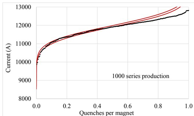
Fig. 7: Training (first quench) in 1000 series and Gaussian fit in the lower half.
