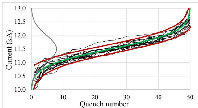
Fig. 3: Example of a Gaussian distribution (grey curve), integral giving training curve for a set of 50 magnets (green curve) with two sigma error (red curves), and 20 realizations of training drawn with a MonteCarlo method (black curves).
