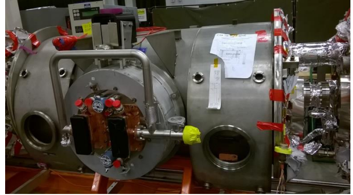
Fig. 6. Picture of the fully assembled cryovault with cavity IA367. The bridging area to the next cryovault is visible on the right side.
