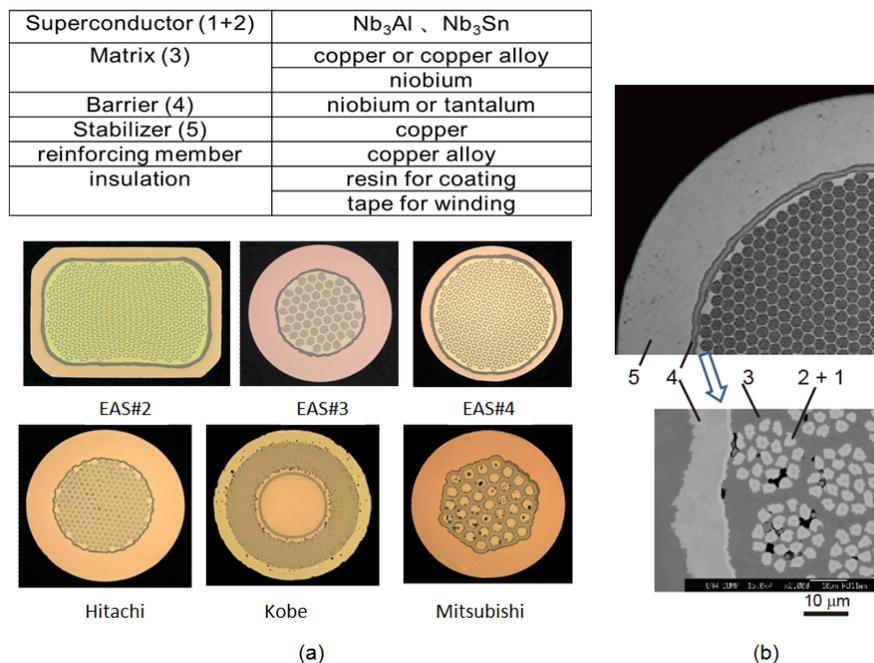
**Fig. 1.** (a) Cross-sectional view of practical Nb<sub>3</sub>Sn wires produced by various manufacturers, (b) the detailed structure of a Hitachi composite wire, where the numerals correspond to those in the table (the lower photo in an enlarged view of a small segment of the upper photo). In the table, the niobium matrix refers to Nb<sub>3</sub>Al wires fabricated by the “niobium tube” and “jelly roll” methods.
