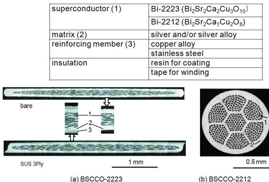
Fig. 2. (a) Cross-sectional views of practical BSCCO-2223 (a) and BSCCO-2212 (b) wires, where the numerals correspond to those in the table.
