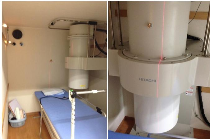
**Fig. 1.** SQUID magnetocardiography (MCG) system MC-6400 operating at University of Tsukuba Hospital.
