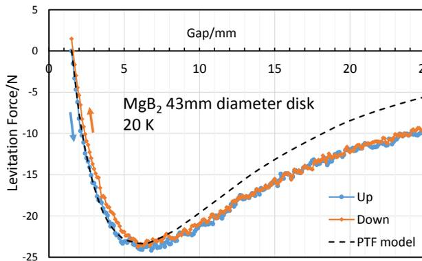
Fig. 5. Hysteresis force curves for a 46 mm diameter, 11 mm thick MgB<sub>2</sub> bulk and PM, field cooled with a 1.5 mm gap at 20 K.
