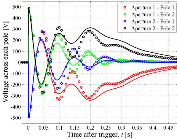
Fig. 3. LHC dipole magnet discharged by a  $2 \times 80$  mF, 500 V CLIQ system and QH covering Aperture 2. Voltage across the four poles, versus time. Comparison between measurement (circles) and simulation (lines).
