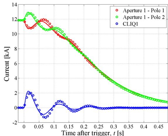
Fig. 2. LHC dipole magnet discharged by a  $2 \times 80$  mF, 500 V CLIQ system and QH covering Aperture 2. Currents in the coil sections and introduced by CLIQ, versus time. Comparison between measurement (circles) and simulation (lines).
