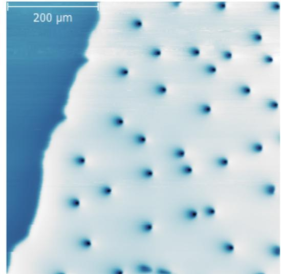
Fig. 1. Scanning SQUID image of vortices near the edge of a YBCO film after field cooling at  $1.47 \mu\text{T}$ . The brightness of each pixel represents the strength of magnetic field at the corresponding point on the sample. The scale bar is  $200 \mu\text{m}$ .
