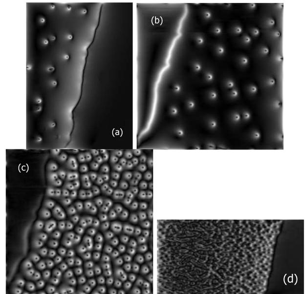
Fig. 2. Current in YBCO film after field cooling at (a)  $0.05 \mu\text{T}$ , (b)  $1.47 \mu\text{T}$ , (c)  $2.10 \mu\text{T}$  and (d)  $5.46 \mu\text{T}$ , calculated from Scanning SQUID images. Brighter regions represent higher currents.
