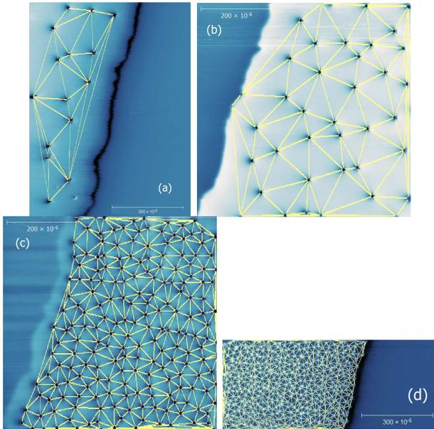
Fig. 3. Delaunay triangulation mapped onto scanning SQUID images at (a)  $0.05 \mu\text{T}$ , (b)  $1.47 \mu\text{T}$ , (c)  $2.10 \mu\text{T}$  and (d)  $5.46 \mu\text{T}$ . Scale bars indicate size in metres. The triangulation is represented by lines connecting each detected vortex position to its neighbours (colour online).
