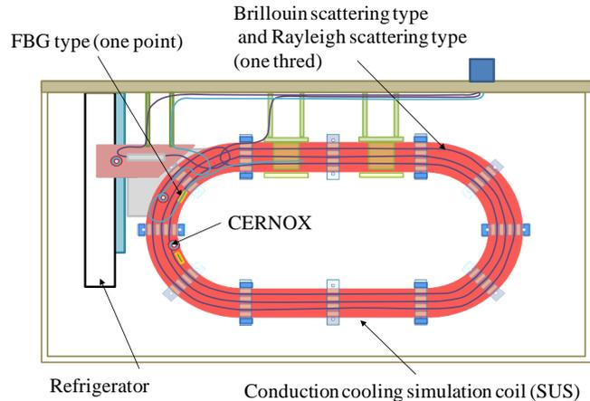
Fig. 3. Thermometry experiment using the thermal simulator
