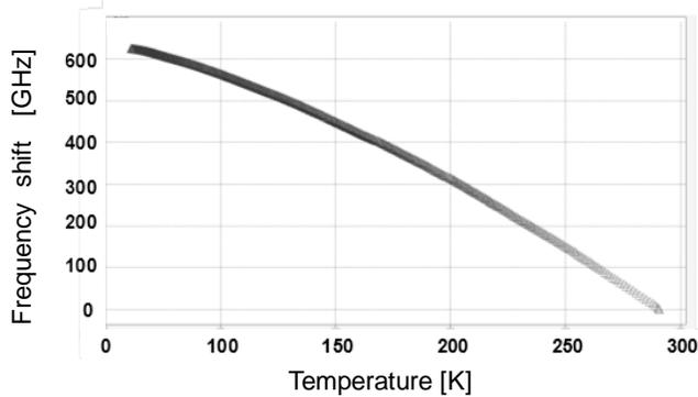
Fig. 6. Temperature and frequency shift at the coil surface measuring point (the Rayleigh scattering type optical fiber sensor)
