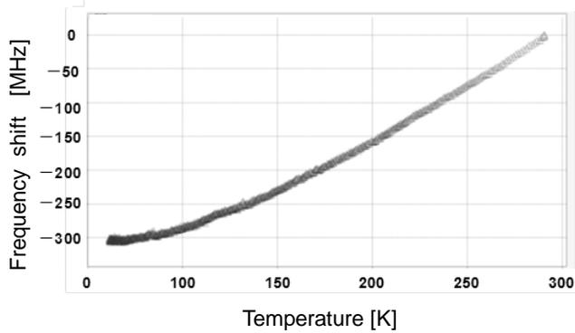
Fig. 5. Temperature and frequency shift at the coil surface measuring point (the Brillouin scattering type optical fiber sensor)
