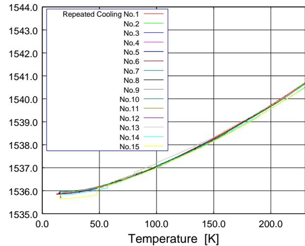
Fig. 7. Temperature characteristics of wavelength for repeated cooling
