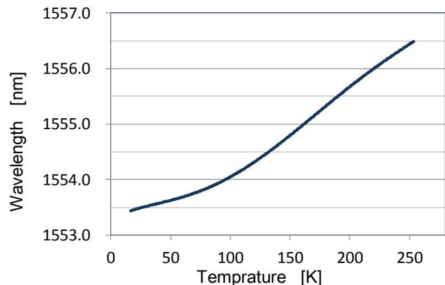
Fig. 10. Temperature characteristics of the wavelength (the combined plating method type optical fiber sensor)
