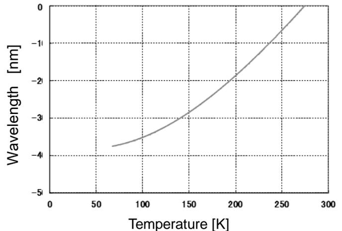
Fig. 4. Temperature and wavelength shift at the coil surface measuring point (the electroplating method type optical fiber sensor)
