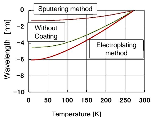
Fig. 2. Temperature and wavelength shift at the FBG part
