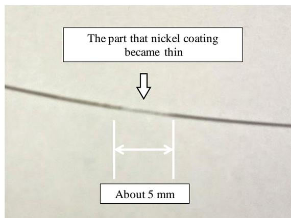
Fig. 11. The rejected prototype of the electroless plating
