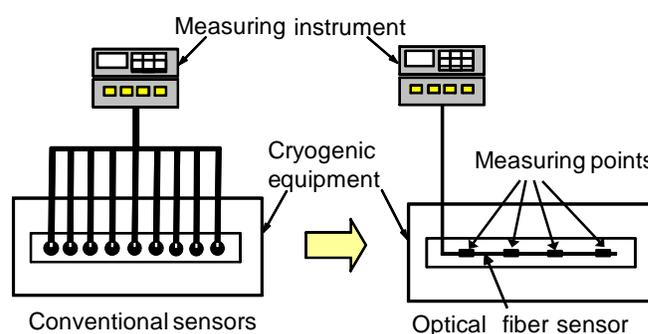
Fig. 1. Conventional sensing and optical fiber sensing
