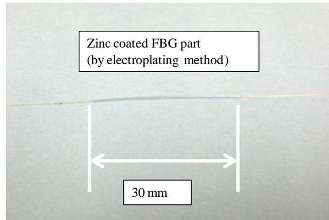
Fig. 9. A temperature detection part of an optical fiber sensor (made by the combined plating method)
