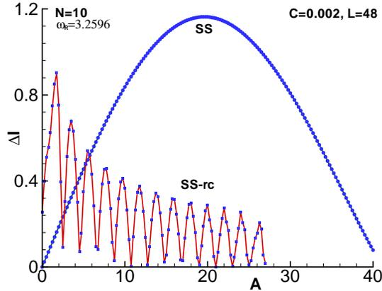
Fig. 4. (Color online) The amplitude dependence of the first SS  $\Delta I$  on the resonance branch (SS-rc) at  $\omega_R = 3.2596$ , compared to the same dependence without shunting (SS).
