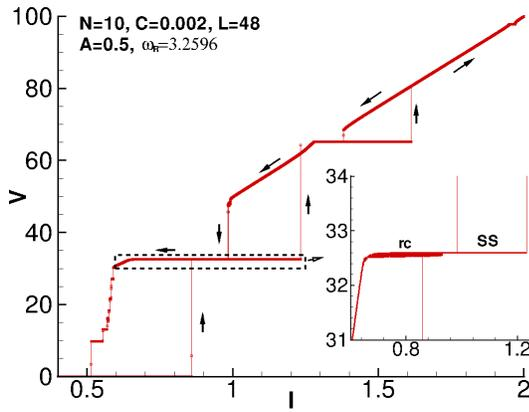
Fig. 3. (Color online) The IV-characteristics of the stack with 10 JJ under external radiation with frequency  $\omega_R = 3.2596$  and amplitude  $A = 0.5$ . Inset enlarges the rc-branch demonstrating Shapiro step on it.
