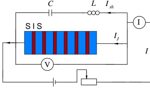
Fig. 1. (Color online) Schema of a stack of JJs with LC shunting elements and the Josephson and the shunt current
